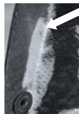
Examples of white marks on the carbon rim of the impact cap.
